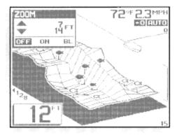
zoom range will be 30 feet. For depths greater than 240 feet the display will only update a 2D view. If the depth range is 480 feet the zoom range will be 30 feet and if the depth range is 600 feet or 1000 feet the zoom range will be 60 feet.
